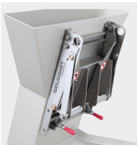
Chutemagnet in sugar production before product inlet
