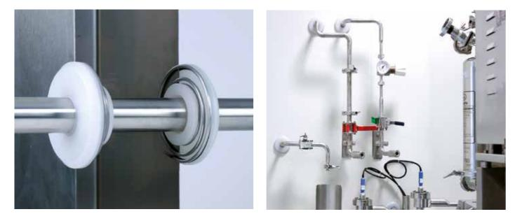
Two seals close the feedthrough according to clean-room standards: the first seal is located on the back of the CleanShut system and provides a seal between the housing and the clean room wall. The second seal is located in the inner passage of the feedthrough and seals it off. This design thus makes using additional sealants unnecessary.
