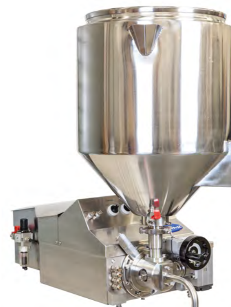
(Below left) heated hopper for hot fills.
