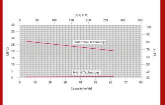
Hybrid technology reduces greatly heat generation in the rear casing region. This benefit is particularly important when pumping low boiling liquids.
