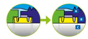
The seal ring adapts to fit perfectly when pressed in, ensuring complete sealing and no dead space
