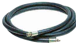
TUBO GOMMA VAPORE (Press. di lavoro 15 Bar-110°C Press. di esplosione 45 Bar-110°C 3/4" (Ø 19x30) - 1" (Ø 25x38)) STEAM HOSE (Working pressure 15 Bar-110°C Explosion pressure 45 Bar-110°C 3/4" (Ø 19x30) - 1" (Ø 25x38))
